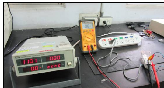
d. 量測 LED 燈泡電流
