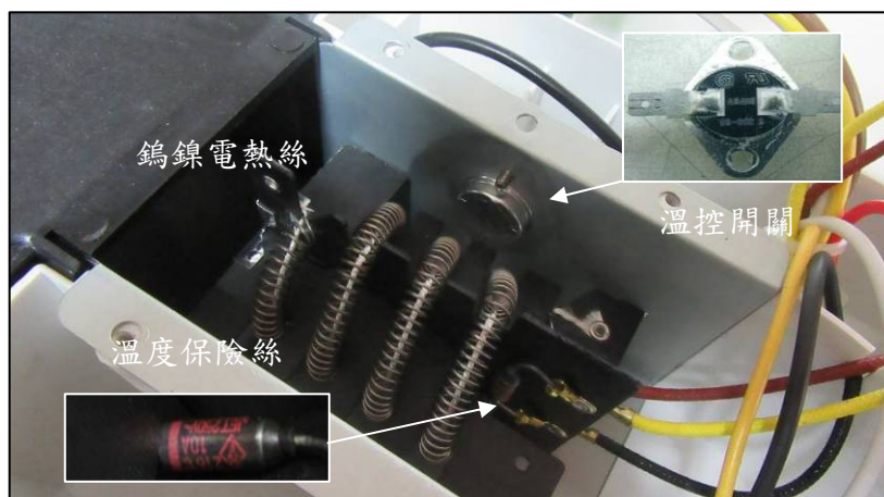
c. 鎢鎳電熱絲的偵測斷電元件—溫度保險絲與溫控開關
